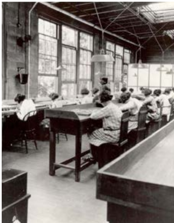
Workers ("radium girls") painting the pointers of luminous dials with radium in the US Radium plant (United States Radium Corporation) in Orange, New Jersey – 1922
